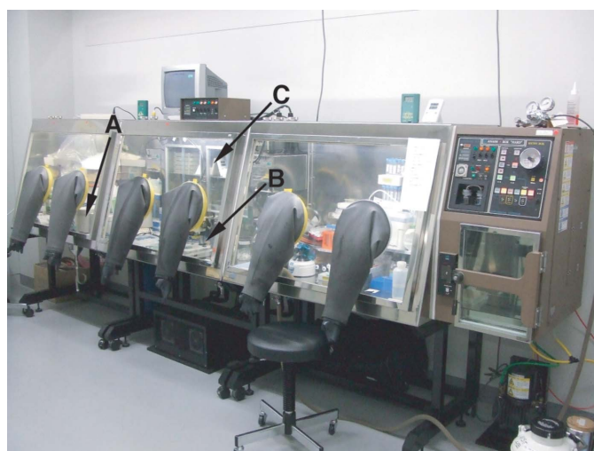
Figure 1 The anaerobic chamber used in the present study. It includes a UV–Vis spectrometer (A), a microscope with CCD (B) and an incubator for crystallization (C) in the anaerobic chamber.
